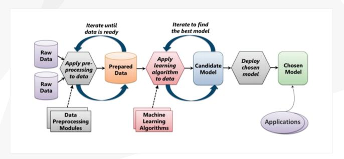
As the above figure illustrates, the whole machine learning process begins with the collection of the raw data. This raw data is not suitable to be used in its present form.
